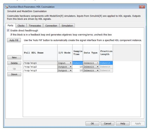
If your model contains purely combinational paths, you can select **Enable direct feedthrough for HDL design with pure combinational datapath** to eliminate the one output-sample delay that occurs with using HDL Verifier blocks and Simulink. For more information on block simulation latency and using the direct feedthrough feature to eliminate it, see "Direct Feedthrough Cosimulation".
