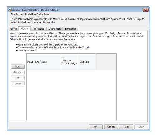
The scrolling list at the center of the pane displays HDL clocks that drive values to the HDL signals that you are modeling, using the deposit method.
