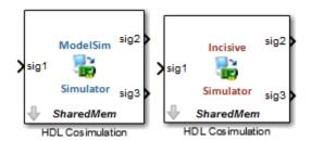
The HDL Cosimulation block cosimulates a hardware component by applying input signals to and reading output signals from an HDL model under simulation in the HDL simulator. You can use this block to model a source or sink device by configuring the block with input or output ports only.
